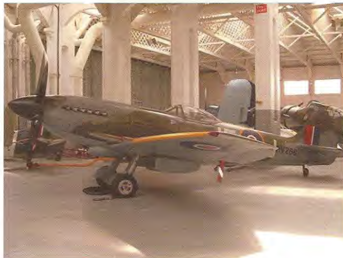
Supermarine Spitfire MV268. This is a RR Griffon engined Mark 14. It is painted up as the aircraft of the late Johnnie Johnson (hence it's code J-EJ) During WW2 JJ was the highest scoring RAF ace and actually flew a Merlin engined Spitfire Mark 9.
