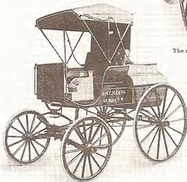
The new style of N. C. R. wagon, showing the sliding base to carry a third register in front.
