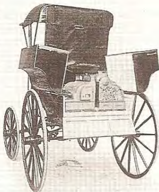
The new style of N. C. R. wagon, showing the arrangement of the hoods.
