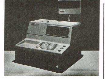
The NCR 210 ECR is a low cost free standing cash register which has been developed around a micro computer system using the INTEL MCS4 logic with a single chip Central Processor Unit. This CPU together with 3 ROMS and 4 RAMS and 3 shift registers each on single plug-in chips provides a small powerful electronic unit contained on one board that can be compared with the TCU, Memory Clock and TIC modules required to perform a similar function on the C280 or C250.
